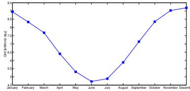
Fig. 2: Global Horizontal Irradiance at the pump station location.
